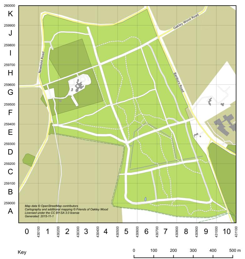
The grid is of 100m squares and is aligned to the OS National Grid (OSGB36). The small numbers are full national grid eastings and northings in meters from the datum. The SW corner of square B0 is at grid reference SP300590, or in full numeric form 430000,259000
